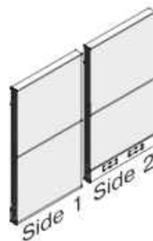
Tile-to-Floor One Side/Standard Base Raceway other Side (optional base power on one side)
