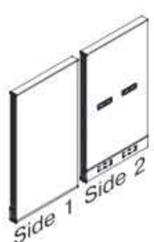
Tile-to-Floor One Side/Standard Base Raceway other Side (beltway power and optional base power on one side)
