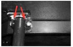
4. Lubricate upper pivot connections for 'endlegs' (Figures 4a and 4b).
