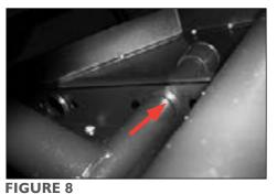
Pivot tubes must be lubricated semi-annually on the table (Figure 8).
