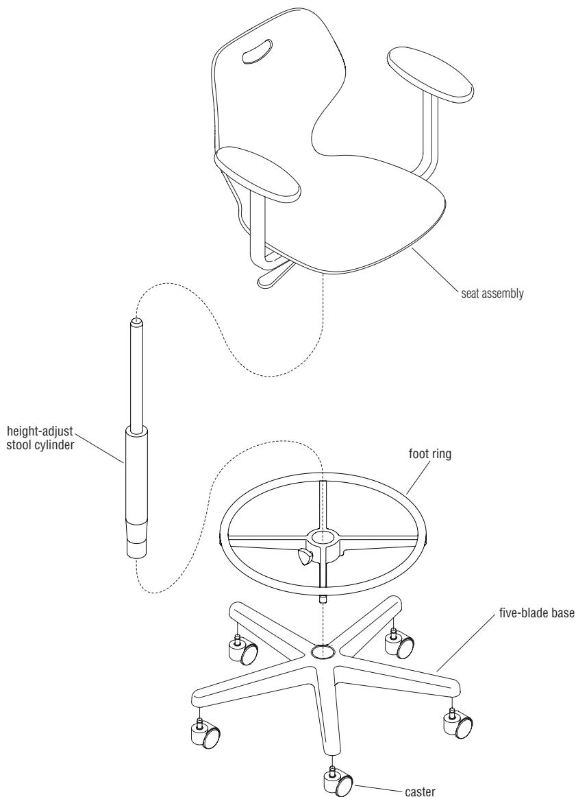
1. With the five-blade base upside-down on a soft protective surface, place the stem of the caster (one at a time) into a mounting hole in the base. Using the spherical-end of a ball-peen hammer, tap the caster between the wheel, and in-line with the metal stem, to drive the caster securely into the base. Repeat with remaining casters and carefully set the base onto the floor.
