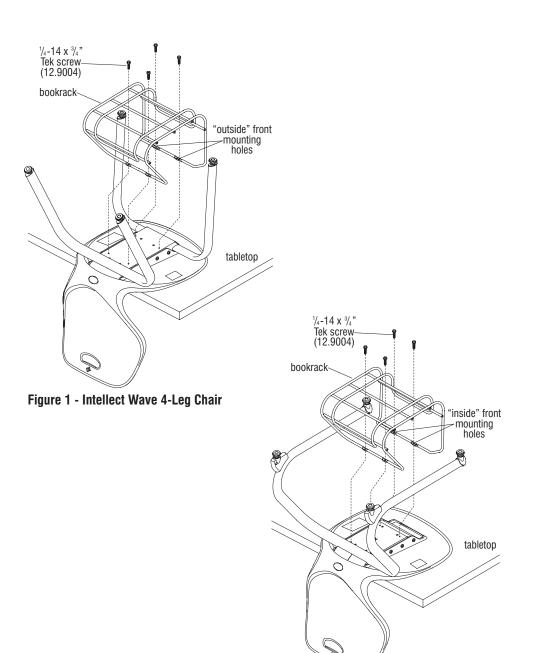
Figure 2 - Intellect Wave Cantilever Chair
